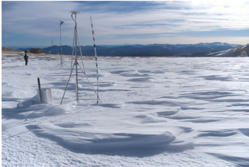
Figure 2. View south-southeast past the GPS installation at Niwot Ridge. The 3-m tall GPS is in the foreground (centre left) along with pole 16. The 5.5-m tall scanning laser is on the left with a person for scale. Sastrugi were not uncommon at the site but are not always present
